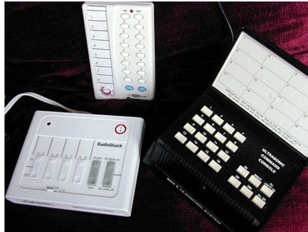
X10 controllers: A simple controller (bottom left), a radio controller (top center), and an original controller (bottom right)
